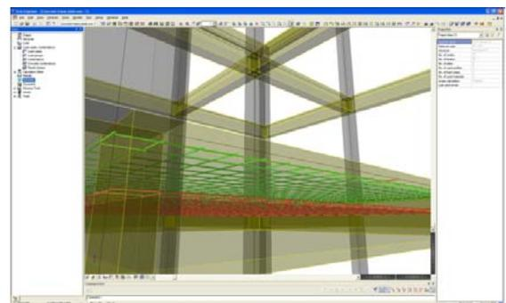
*Structural work model in Scia Engineer
