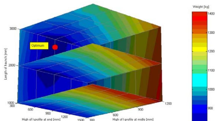
An optimal shape of the tapered beam was determined.
