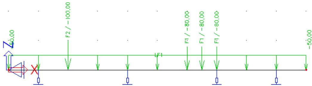
The user can set the limits to move the supports, each variant is calculated and reactions are evaluated. The goal function can be a simple formula, which calculates the sum-of-squares of deviations from an average value of reaction.
